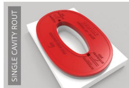
insertion at one of the notches in the jig as there is a larger opening in these areas. Plunge the router down into the foam, then move the router in a clockwise direction around the inside of the jig. Resulting cut is always offset a 1/16" away from the jig.
