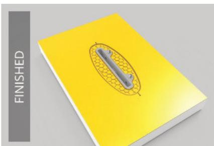
Once the board has been hot coated and has cured it is time to sand the board and boxes. The shape of the dam on the box creates a raised area that needs to be sanded down flush with the bottom surface of the board.
